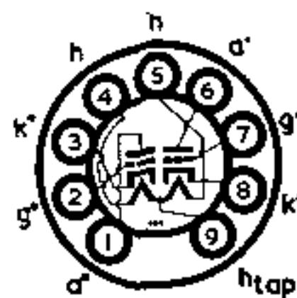
The BRIMAR 6057 is a trustworthy miniature double triode with separate cathode connections and a tapped heater enabling it to be used in a variety of applications.
